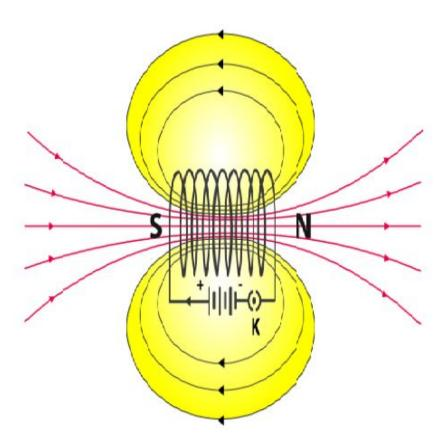
When the north pole of the bar magnet is brought close to the end connected to the negative terminal of the battery, the solenoid repels the battery. As like poles repel each other, we can infer that the end connected to the negative terminal behaves as a north pole while the end connected to the positive terminal behaves as a south pole.
